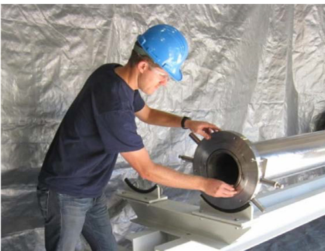
The SCWO (Super Critical Water Oxidation) has recently undergone factory acceptance testing before shipping to BGCAPP.
