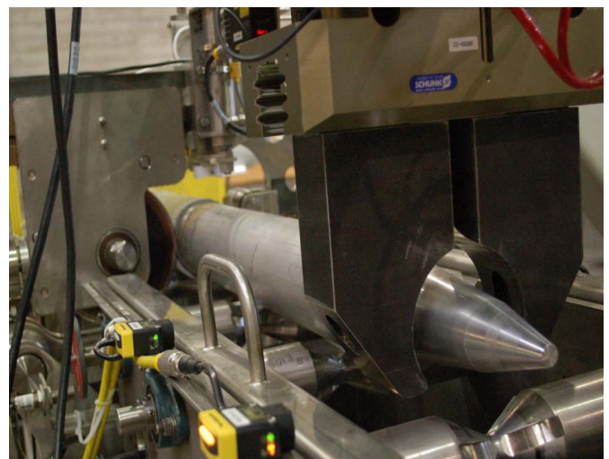
The rocket cutting and rocket shear machine have joined other BGCAPP specific equipment at the construction site.
